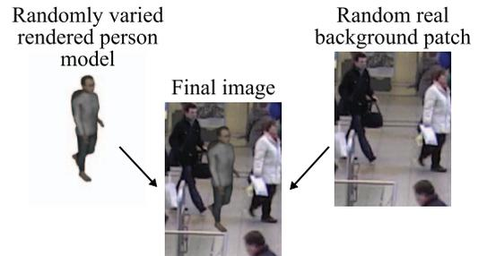
**Fig. 2:** The 3D model is varied randomly and passed on to the OpenGL renderer. The output is merged with a randomly chosen background patch in the image composition stage.
